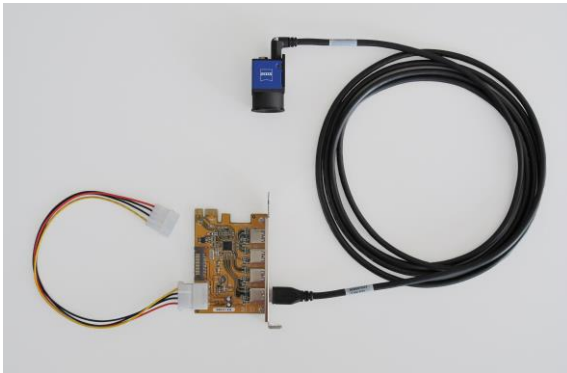
Molex power connector cable, PCIe interface card, USB 3.0 cable, camera
